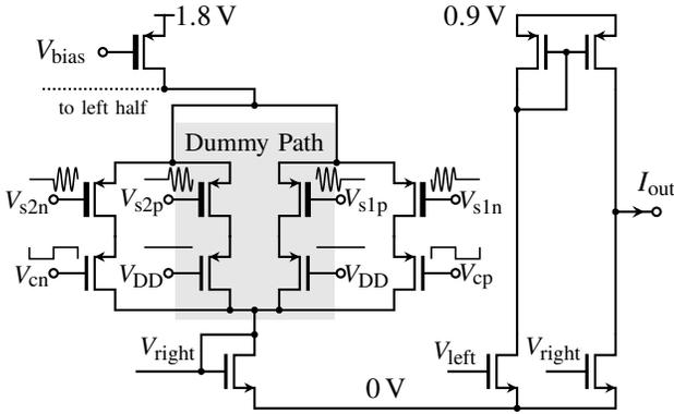
Fig. 2: Implementation of the Charge Pump (right half)
