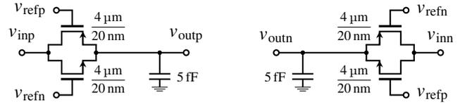
Fig. 3: Implementation of the sub-sampling phase detector
