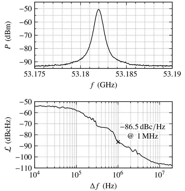
Fig. 6: Measured Spectrum (top) and Phase Noise (bottom) of the LC Oscillator. RBW = 500 kHz (power) / 10% (phase noise), VBW = 500 kHz, Attenuation = 0 dB
