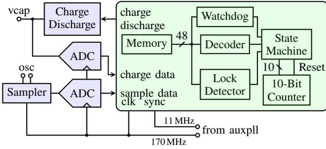
Fig. 7: Implementation of Automatic Frequency Calibration and Lock Assist; Green: Digital, Blue: Analog
