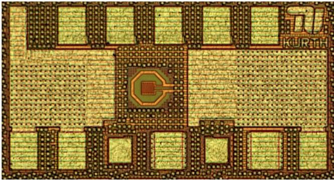
Fig. 5: Die Photograph of the LC Oscillator
