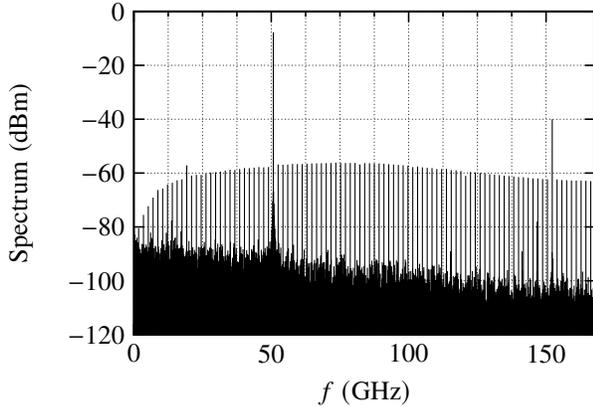
Fig. 8: Simulated output spectrum of the entire SSPLL in lock at 50.75 GHz (number of points: 1920)
