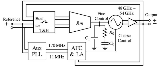
Fig. 1: System Architecture of the Sub-Sampling Phase-Locked Loop including the main phase control loop and the frequency calibration/lock assist (AFC & LA) with auxiliary PLL
