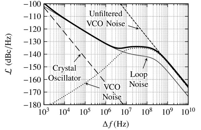
Fig. 9: Calculated/simulated phase noise spectrum of the entire SSPLL in lock (based on simulation data and models as well as measurement results of the LC oscillator)
