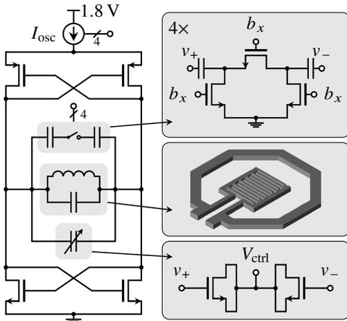
Fig. 4: Top-level Circuit of the LC Oscillator
