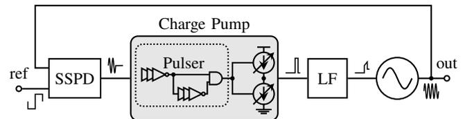
Fig. 1: Typical SSPLL system architecture with annotated associated signal waveforms and the implementation of the charge pump with a pulser (gray box)
