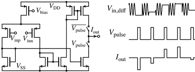
Fig. 2: Circuit implementation (left) and signals (right) of a conventional charge pump in a sub-sampling phase-locked loop
