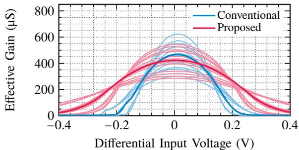
Fig. 4: Simulated effective charge pump gain against input voltage with inclusion of process and temperature variations. The typical corner is emphasized
