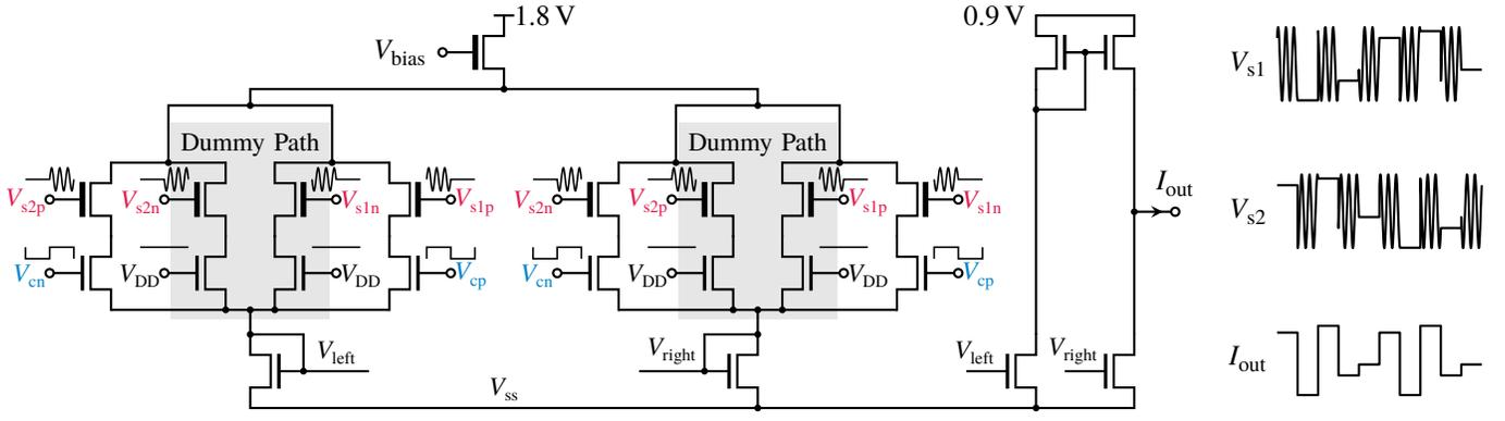
Fig. 3: Top-level circuit implementation of the novel SSPLL charge pump (left) and corresponding timing diagram (right)
