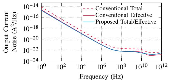
Fig. 6: Simulated total/effective output current noise of the conventional and the proposed SSPLL charge pump
