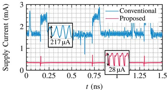
Fig. 5: Simulated supply current consumption of the conventional and the proposed SSPLL charge pump
